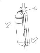
Replace the new battery and install the cover back.
