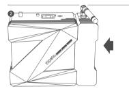
2 | Align connector of Zipabox EnOcean Expansion Module to expansion Slot 2 of Zipabox (or to module connected into Slot 2)
